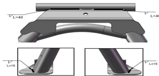
Gambar 7. Ilustrasi proses *Welding Permanent 2*
