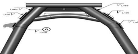
Gambar 5. Ilustrasi proses *Welding Permanent 1*
