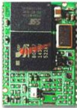
Gambar 6. *Bluetooth module* MB-C04
